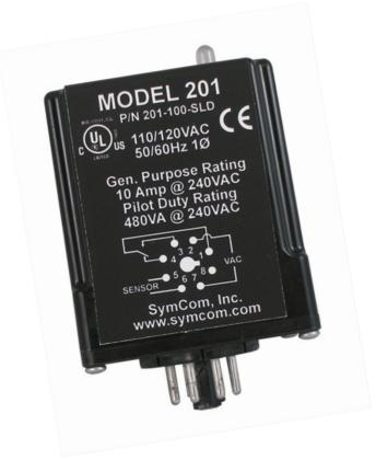
The MotorSaver® Model 201-100-SLD is an 8-pin plug-in style seal leak detector to sense seal failures on submersible pumps. The unit plugs into an OT08-PC or RB08-PC octal socket (sold separately).
